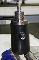
4. Once the gland has been unscrewed all the way, remove the cylinder from the vise. If necessary, apply low pressure air to the head end of the cylinder housing to dislodge the gland from the cylinder barrel as shown below:
