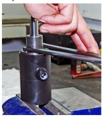
7. Stamp the base of the assembled cylinder with the letters 'SS' to indicate that it is now a short-stroke cylinder.
