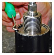
2. Secure cylinder housing in a vise, threaded rod-end up, as shown.
